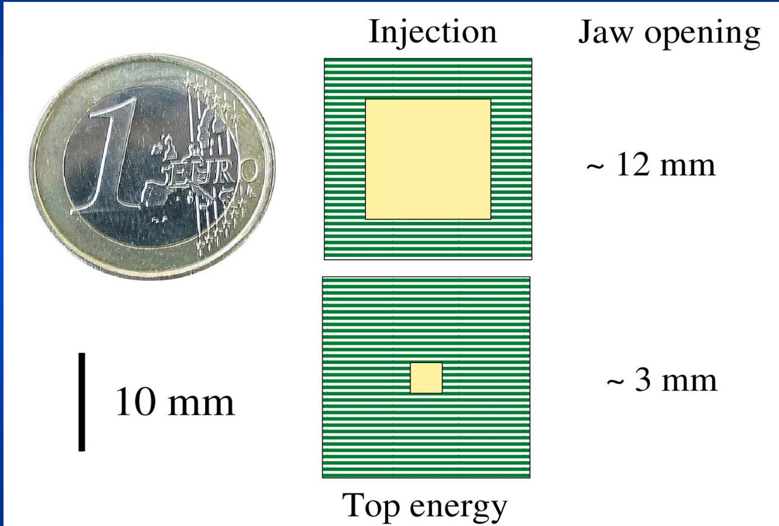
*LHC beam will be physically quite close to collimator material and collimators are long (up to 1.2 m)!*
