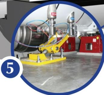
A new longitudinal restraining system is being fitted to 50 quadrupole magnets
