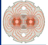
The LHC has a circumference of **26.7** km, with 20km filled with superconducting magnets operating at 8.3 T. The refrigerators producing the liquid helium to cool the magnets consume **40 MW** of power.
