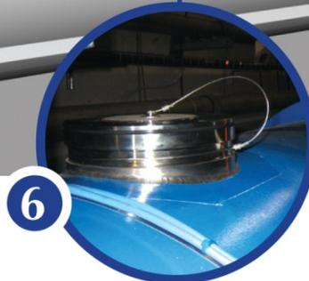
Nearly 900 new helium pressure release ports are being installed around the machine
