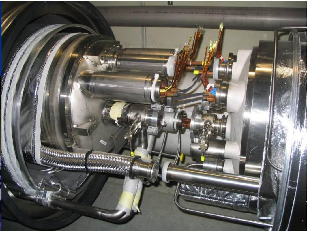
During cool-down of the LHC the machine contracts by **80 metres, 10m per octant**
